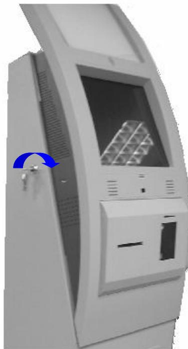
Fully pull out the front bezel in the direction indicated after unlocking the device.
